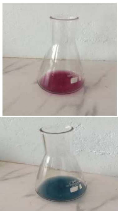
Figure 3: wine red colour of solution changes to pale blue at the end point
