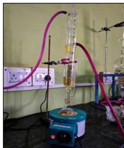
Figure 10: Soxhlet Extraction of Tridax procumbens
