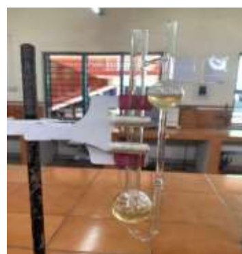
Fig no:7 Determination of viscosity Determination of Surface Tension using Stalagmometer (Drop Count Method):
