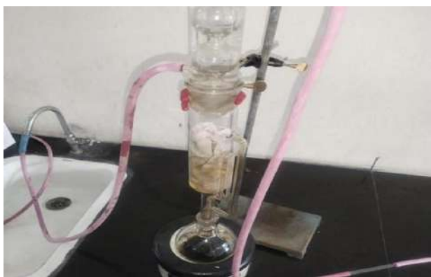
Fig 4: Soxhlet extraction for ethanolic extract
