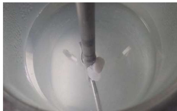
Figure 11: Floating pulsatile release tablet during dissolution
