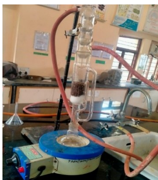
Figure 3: Extraction by using Soxhlet Apparatus
