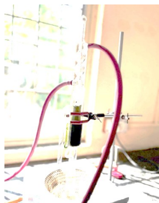
Figure 3: Assembly of Soxhlet Extraction
