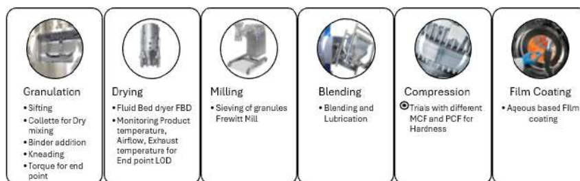
Figure 2: Process Flow of Drug product manufacturing
