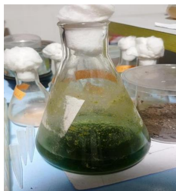
Fig.1. Sample kept after adding n-hexane, methanol and caustic soda
