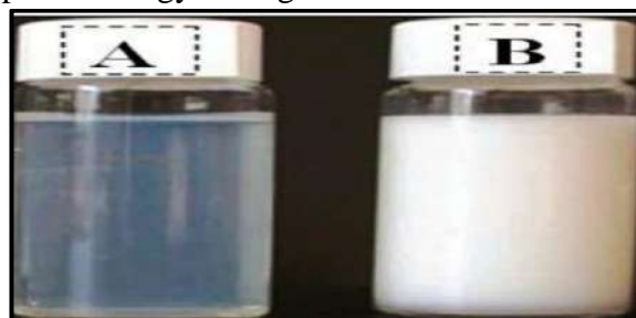
Fig. 1: (A) Nanoemulsion and (B) Macroemulsion With Droplet Diameters of Less Than 100 Nm and More Than 1000 Nm, Respectively 5
