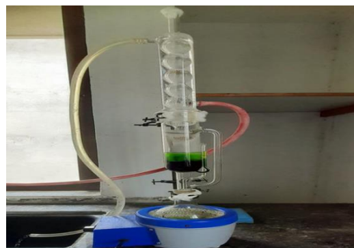
Fig 2: Soxhlet Extraction Of Tridax Procumbens
