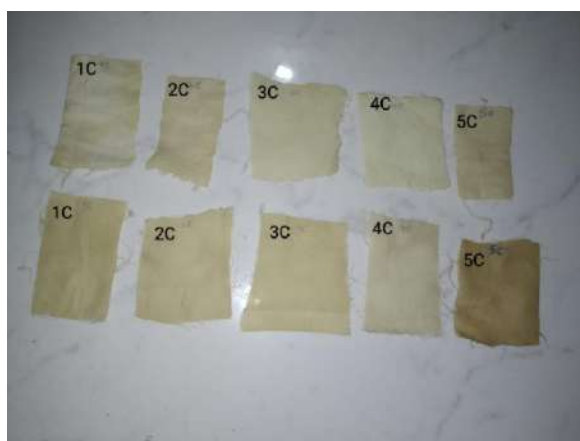
Fig. No. 6. Rubbing fastness property of samples 'C' (upper samples 30 mins. And lower samples 31 hrs)
