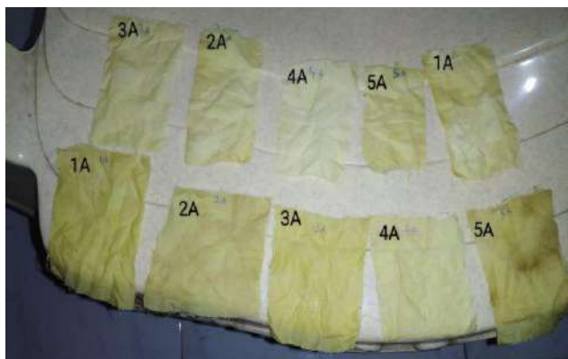
Fig. No. 3. Washing fastness (wet) samples 'A' (upper samples 30 mins. And lower samples 31 hrs)
