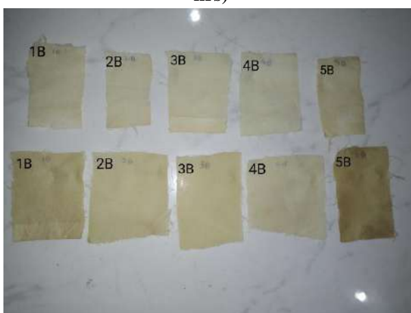
Fig. No. 5. Light fastness property of samples 'B' (upper samples 30 mins. And lower samples 31 hrs)
