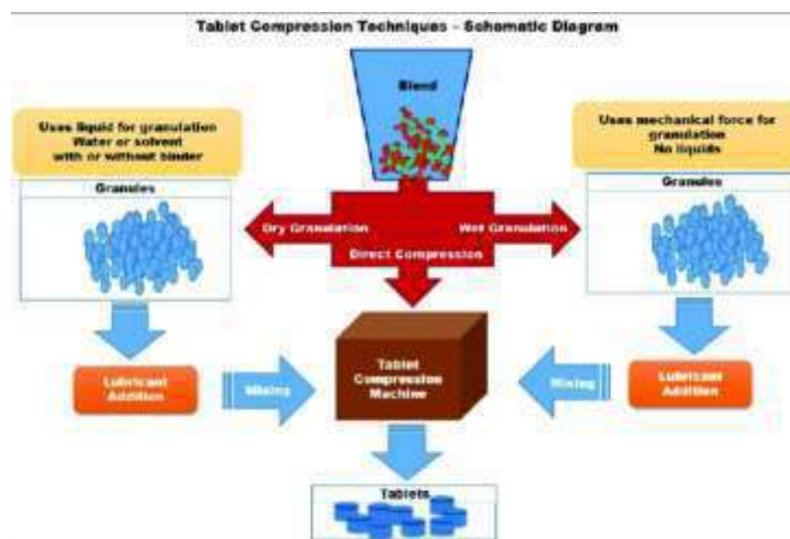
Fig no 2: Schematic illustration of matrix tablet formulation steps—mixing, granulation, and compression process.
