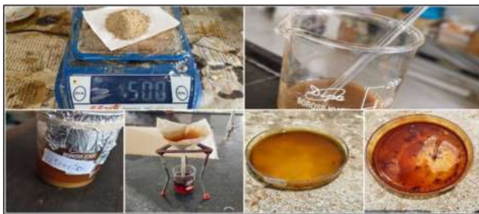
Fig No:-05 Extraction process by maceration
