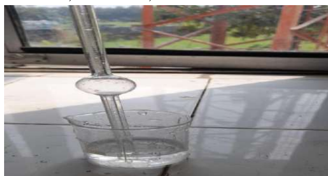
Fig 10: Stalagmometer for surface tension determination
