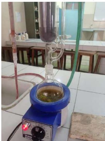
Fig 5. Extraction Of Crude Drug With Soxhlet Apparatus
