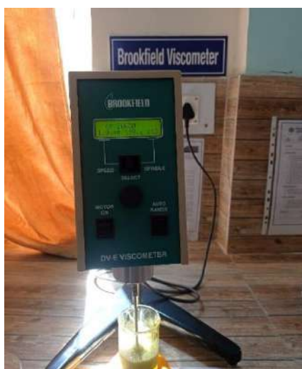
Figure 15. Evaluation Of Viscosity Of Emulgel With Brookfield Viscometer
