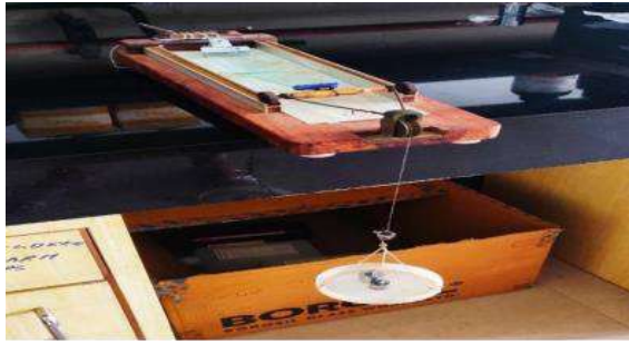
Fig.no.2 Instrument for testing Spreadability
