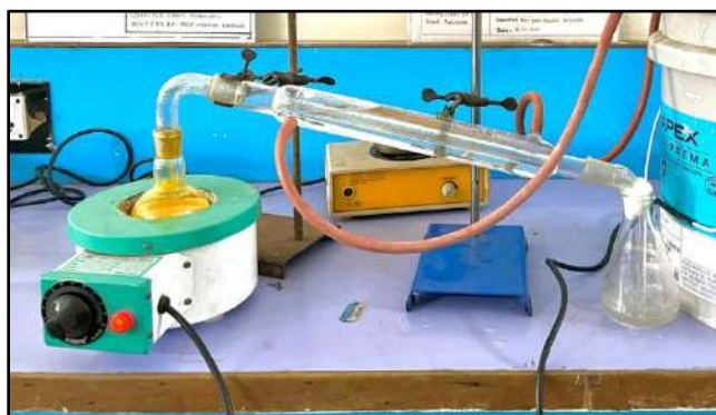
Fig. 09 Extraction Using Steam Distillation
