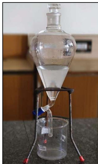
Fig. 10 Phase Separation using Separating Funnel Clove Essential Oil:
