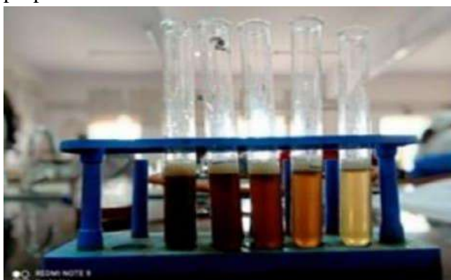
Fig 7 Foaming ability and foam stability test
