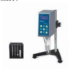
Brookfield viscometer is used to measure the viscosity of scrub.
