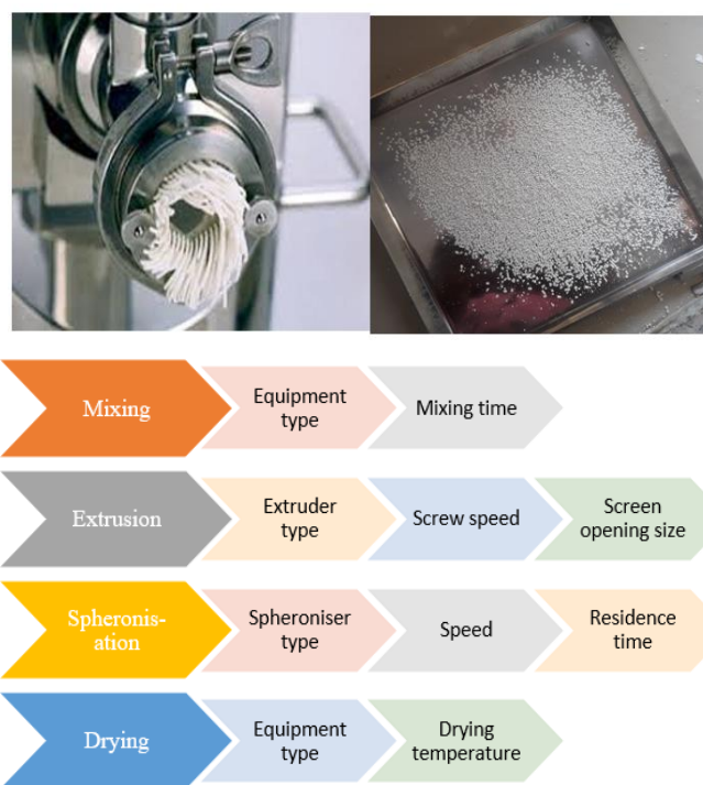
Fig. 1.2. Processing flowchart indicating individual process variables (18)
